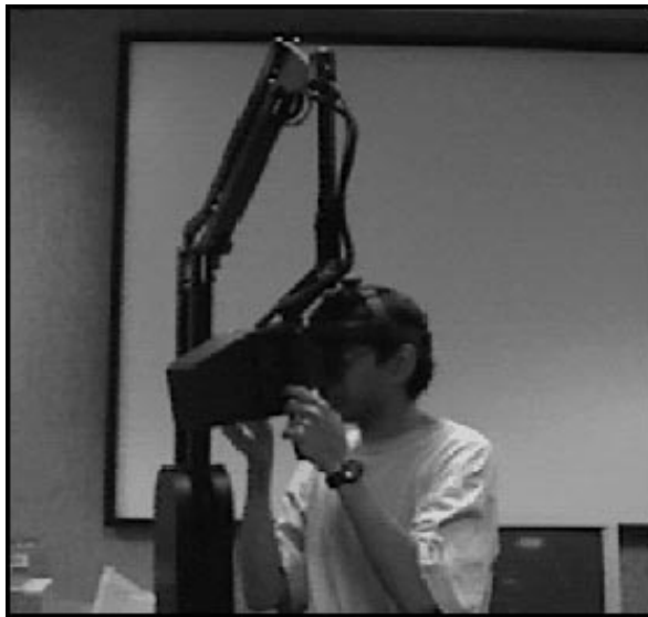
Figure 1.20 In IV, a remote viewer is able to walk through and observe a scene from anywhere using virtual reality devices such as a head-mounted display or a boom.
